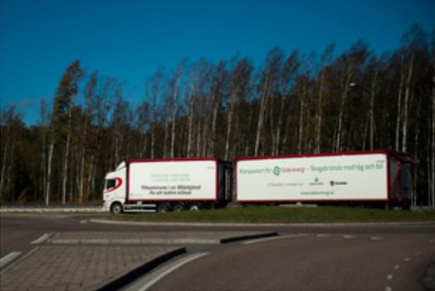
Sweden has longer and heavier vehicles than do the rest of Europe. Through the European Modular System, combinations of existing loading units into longer and heavier vehicles are used, allowing vehicle combinations of a length of 25.25 meters and a weight of 60 ton. High capacity vehicles reduce fuel consumption, greenhouse gas emissions and costs.
