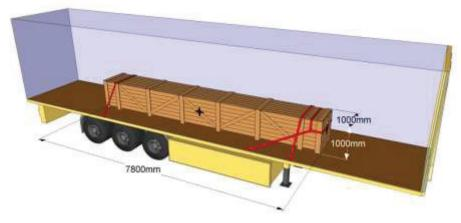
The trailer has an ordinary plyfa floor that is swept clean and is free from frost, ice and snow. The trailer is built in accordance with the EN 12642 standard, XL class, and the lashing points on the trailer are designed in accordance with the EN 12640 standard, each with a lashing capacity (LC) of 2000 daN. The transverse distance between the lashing points is about 2.4 m.
