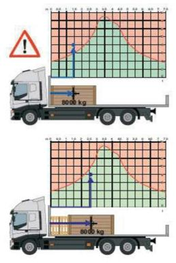
Generally, the maximum pay load may be used only when the centre of gravity is positioned within narrow boundaries about half the length of the loading space.
