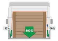
In case of deformable cargo, these high local forces will cause a deformation of the cargo, thus freeing space for the cargo to move, comparable to the movement of the cargo due to the elongation of a strap.
