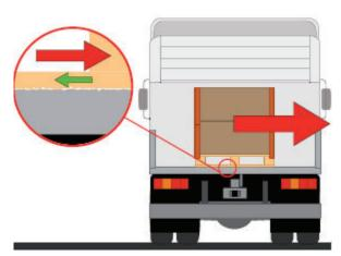
Centrifugal forces are the forces acting on the vehicle and its load at cornering. They tend to push the vehicle and its load to the outside of the turn. The centrifugal force is calculated using the formula below:
