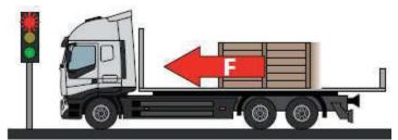
Deceleration forces; when braking, the load tends to slide forward
