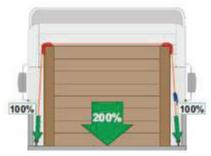
The use of large corner protectors can contribute to the distribution of lashing forces over a greater zone and thus to the reduction of the movement of the cargo.
