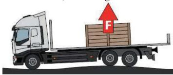
Buoyancy forces; shocks, vibrations and oscillations generate inertial forces that result in the load losing contact with the platform of the vehicle
